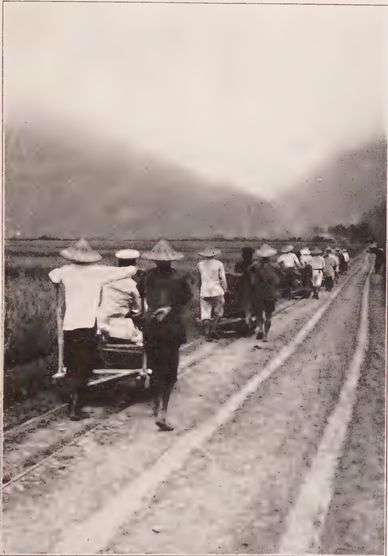
In Formosa are miles of push-car railways, carrying both passengers and goods, and operated by Chinese labourers. The natural resources of this island, acquired from China, have proved of great value to Japan
